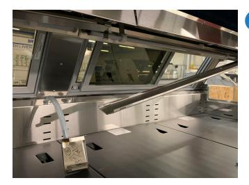
Don't panic! When cleaning or merchandising the case, it is possible that either the catch pan, drip rail or both can be knocked loose. It is very easy to reinstall each item and you can be back on track within a matter of minutes. The most important thing to remember is ensuring each part is attached correctly into the provided clips.
