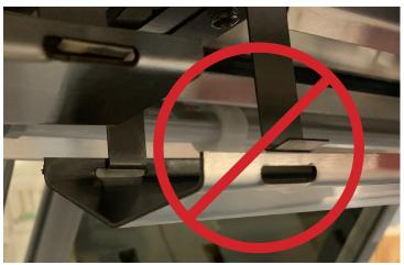
The front clip did not get inserted in the slot on the drip rail, this could cause the water to not drain properly from the drip rail.
