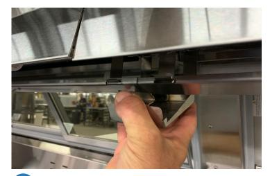
4 Attached the catch pan by clipping it over the front and back of the end of the drip rail. The end with the hose should be at the back of the case.
